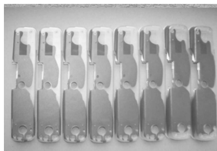
Fig. 6 Range of multi color molding (1/10/50100/150...)
